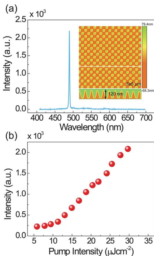
**Fig. 6** (a) Laser action from a two-dimensional DFB structure. The inset shows AFM images of two dimensional DFB structures. (b) Output intensity as a function of the pump fluence, indicating a pump threshold of about  $10 \mu\text{J cm}^{-2}$ .
