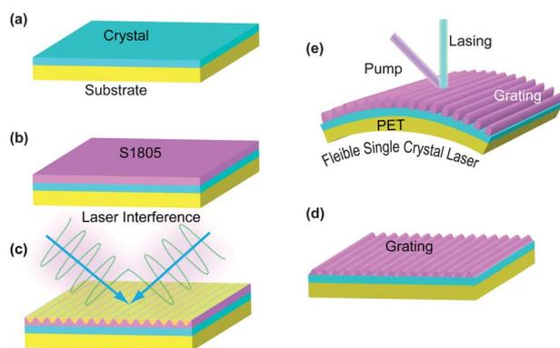
**Fig. 3** The fabrication process of the crystal DFB laser. (a) Laminate the grown crystal onto the substrate. (b) Spin-coat the photoresist onto the crystal layer. (c) Laser interference pattern the resist. (d) Development of the photoresist. (e) A schematic illustration of a flexible crystal laser device.
