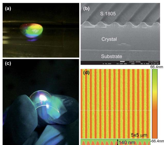
**Fig. 4** (a) Iridescence color caused by the diffraction of the fabricated grating could be observed from a sample device. (b) The SEM image of a side view of the device with one-dimensional (1D) grating. (c) A photograph of an experimental flexible single-crystal laser device. UV illumination is used to show the devices fluorescence. (d) AFM images of a one dimensional DFB structures. The period is about 330 nm, the modulated depth is more than 100 nm.
