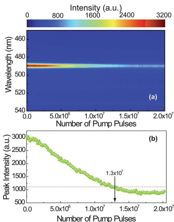
**Fig. 8** (a) A photostability test for an operating 1D DFB crystal laser, (a) spectral evolution and (b) peak intensity as a function of the number of pump pulses.
