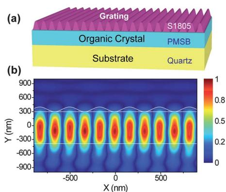
**Fig. 2** (a) The design of the crystal distributed feedback waveguide laser. (b) The Eigen modes (electric field energy) of the DFB design with the grating fabricated on top of the continuous crystal waveguide.
