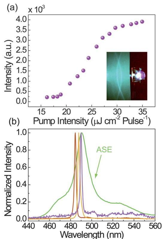
**Fig. 5** (a) Output intensity as a function of the pump fluence, indicating a pump threshold of about  $18 \mu\text{J cm}^{-2}$ . The inset shows photographs of an operating BSB-Me crystal one-dimensional DFB laser. (b) The light-emission spectrum from BSB-ME in the presence of ASE and laser action from three different DFB grating periodicities.
