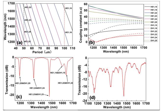
Fig. 2. (a) Relationship of the grating period and the resonant wavelength of different high-order cladding modes (HE1,15 and HE1,16 correspond to the first-order diffraction, HE1,22 ~ HE1,25 correspond to the second-order diffraction). (b) Coupling constants of different high-order cladding modes with the wavelength range of 1200 ~ 1700 nm. (c) Theoretically simulated transmission spectrum. (d) Typical transmission spectrum of the LPFG with a period of 100  $\mu$ m.
