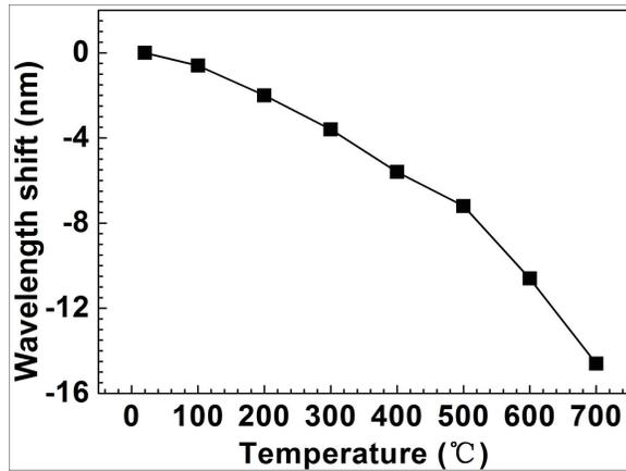
Fig. 3. Shift of the loss peak wavelength of the LPFG with temperature.
