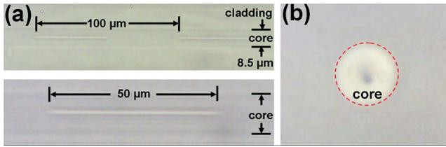
Fig. 1. (a) Side-view microscope image of RI modulation region in the fiber core. (b) Cross-section microscope image of RI modulation region in the fiber core.
