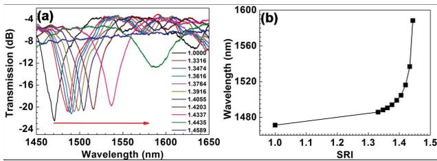
Fig. 4. (a) Transmission spectra of LPFG with different RI solutions. (b) Shift of the loss peak wavelength of the LPFG with different RI solutions.
