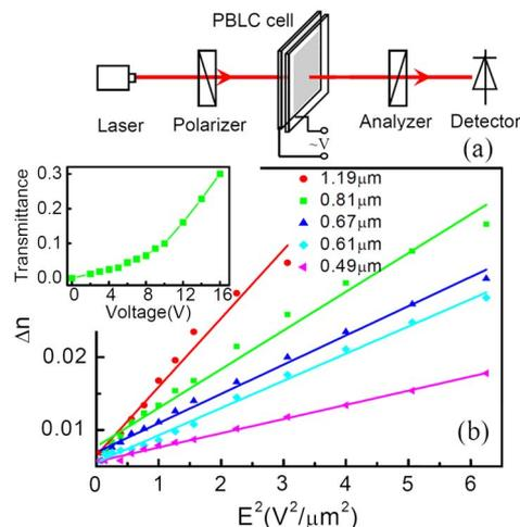
Fig. 1. (Color online) The field-induced birefringence measurement of PSLCs. (a) The schematic experimental setup. (b) The voltage-birefringence curves for the samples with different chiral pitches. The inset shows the voltage-transmittance curves of PSLCs of  $0.81 \mu\text{m}$  pitch.
