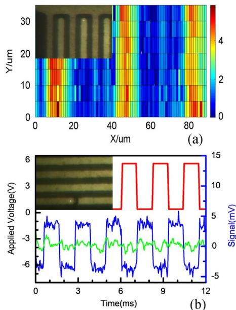
Fig. 4. (Color online) The electro-optical measurement of interdigital electrodes. (a) The measured two-dimensional electric distribution. (b) The measurement of an electrode with open defects. The upper curve is the applied voltage, and the lower curves are the signals measured on each side of the broken line. The insets of (a) and (b) are the interdigital electrodes with their finger and spacing of  $10\ \mu\text{m}$ .
