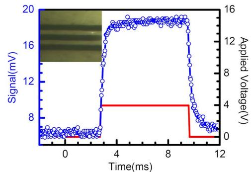
Fig. 3. (Color online) The typical data of the electro-optical probe experiment. The solid line is the applied electric signal to the line of the coplanar waveguide, and the circle-dot line shows the modulation light intensity read by a photodiode detector. The inset is the measured circuit and the spot of the probing beam monitored by a camera.
