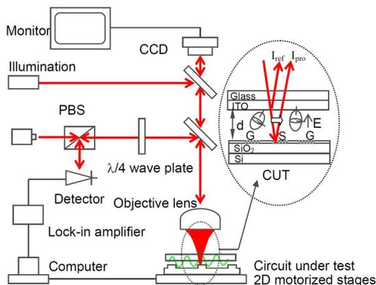
Fig. 2. (Color online) The schematic electro-optical system based on PBLCs. The inset shows the probe configuration.
