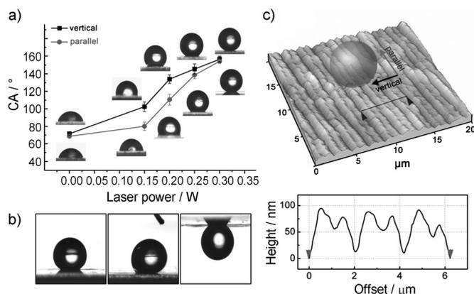
Figure 3. a) Dependence of the CA on the laser power in both vertical and parallel directions of the grating structure. Photographic images of a water droplet on the different substrates have been inserted. b) Images of a water droplet on a flat and tilted biomimetic graphene surface. Tilt angles (from left to right) are 0°, 45°, and 180°, respectively. c) 3D-AFM image of the biomimetic graphene substrate and the corresponding height profile plot.
