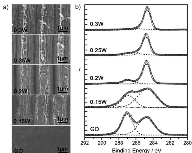
Figure 2. a) SEM images of the grating structure of the graphene surface fabricated at different output power. b) C1s XPS spectra of pristine GO and GO films after two-beam laser interference treatment at different laser power. The spectra have been offset along the vertical axis for clarity.
