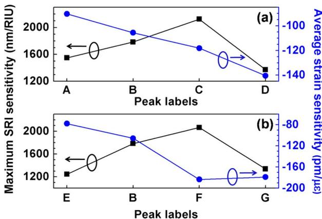
Fig. 9. Maximum SRI sensitivities and average axial strain sensitivities of the peaks A–F.
