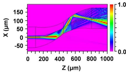
Fig. 3. Simulated light propagation in the SFT with total length of 700  $\mu\text{m}$ , axial offset of 114  $\mu\text{m}$ , and taper waist diameter of 65.0  $\mu\text{m}$ , respectively, at the input wavelength of 1.55  $\mu\text{m}$ .
