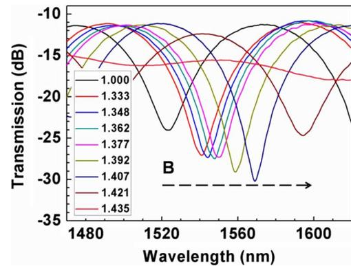
Fig. 5. Transmission spectrum of peak B changes with different SRI. The numbers denote to the SRI values.
