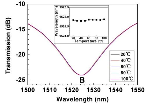
Fig. 4. Transmission spectrum of peak B changes with different temperature. Inset: wavelength of peak B changes with temperature.
