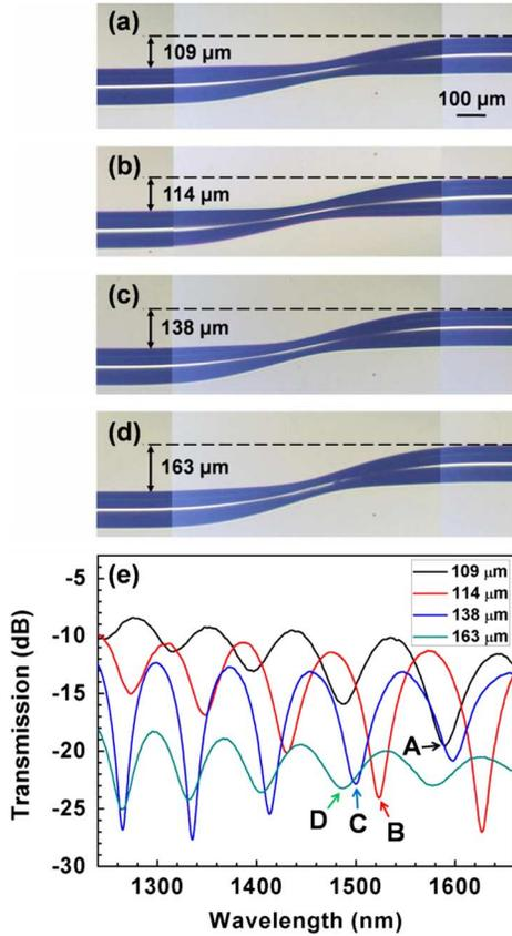
Fig. 1. (a)–(d) Optical microscope images of the SFTs with different axial offsets when the taper waist diameters are fixed to  $65\ \mu\text{m}$ . (e) Transmission spectra of the SFTs corresponding to (a)–(d).
