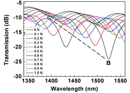
Fig. 7. Transmission spectrum of peak B changes with different axial tension.
