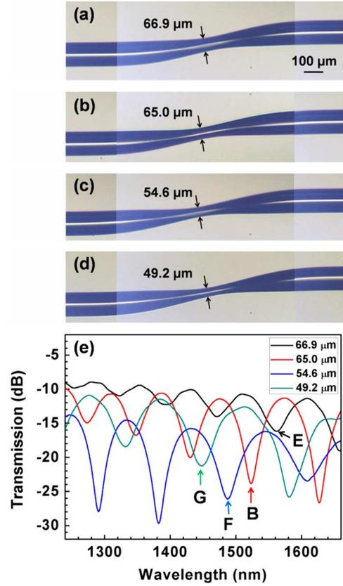
Fig. 2. (a)–(d) Optical microscope images of the SFTs with different taper waist diameters when the axial offsets are fixed to  $114\ \mu\text{m}$ . (e) Transmission spectra of the SFTs corresponding to (a)–(d).
