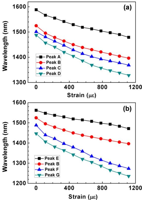
Fig. 8. Wavelength of attenuation peaks A–F shift as a function of axial strain. Peaks in (a) and (b) belong to the SFTs with different axial offsets and taper waist diameters, respectively.
