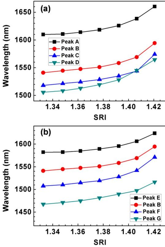
Fig. 6. Wavelength of attenuation peaks A–F shift as a function of SRI. Peaks in (a) and (b) belong to the SFTs with different axial offsets and taper waist diameters, respectively.
