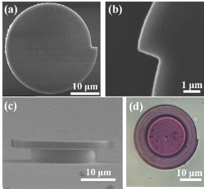
Fig. 1. (a) The top view SEM photograph of the microdisk; (b) the local and amplifying view SEM of the microdisk; (c) the side view SEM photograph of the microdisk; (d) the optical microscope image of the microdisk.
