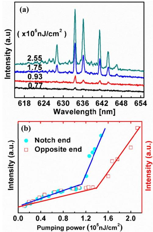
Fig. 2. (a) The measured spectra of the spiral-shaped microcavity with a notch size of  $1 \mu\text{m}$  for five different pumping powers; (b) the measured signal intensities of the output from the notch and the opposite direction versus the power of the pump laser.
