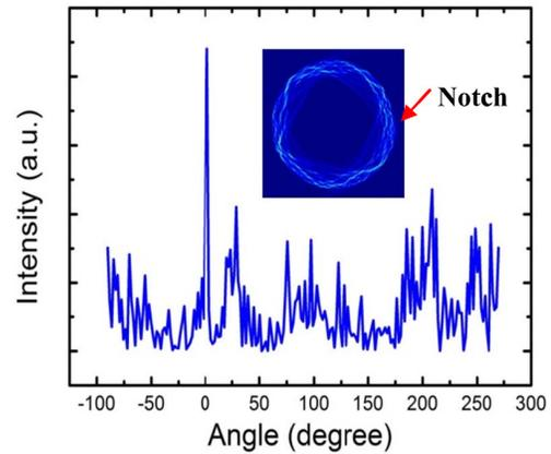
Fig. 4. FDTD simulation results of spectral mode structure. Inset: the intensity distribution of the mode at 631.65 nm.
