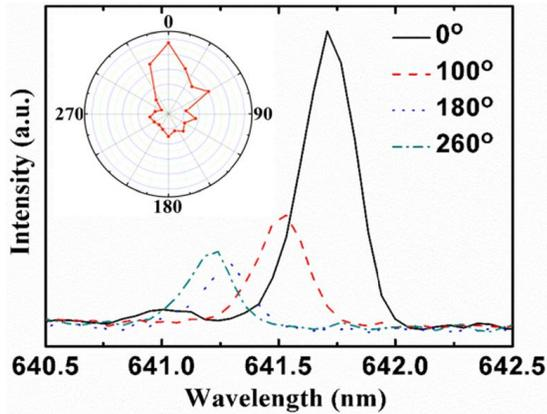
Fig. 3. The emission spectra of the spiral-shaped microdisk cavity laser at room temperature. Inset: the lasing intensity distribution measured with the signal emitted from different angles.
