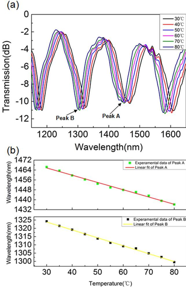
Fig. 3. (a) Transmission spectra of the magnetic fluid-sealed OMT under different temperatures. (b) Relationships between temperature and wavelength shift of the resonant peaks.
