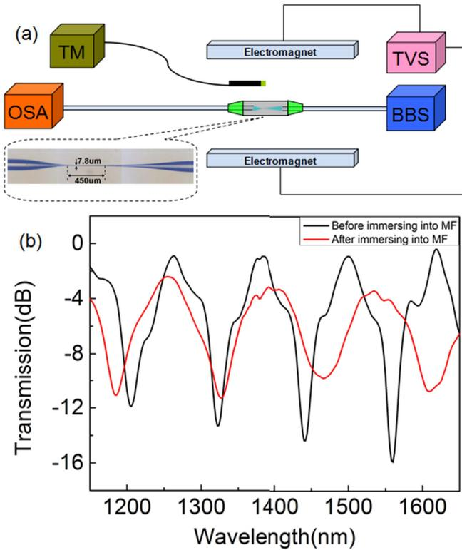
Fig. 1. (a) Experimental setup for the magnetic field sensing. The inset shows optical microscope image of the OMT. (b) Transmission spectra of the OMT before and after immersing in the ferrofluid.
