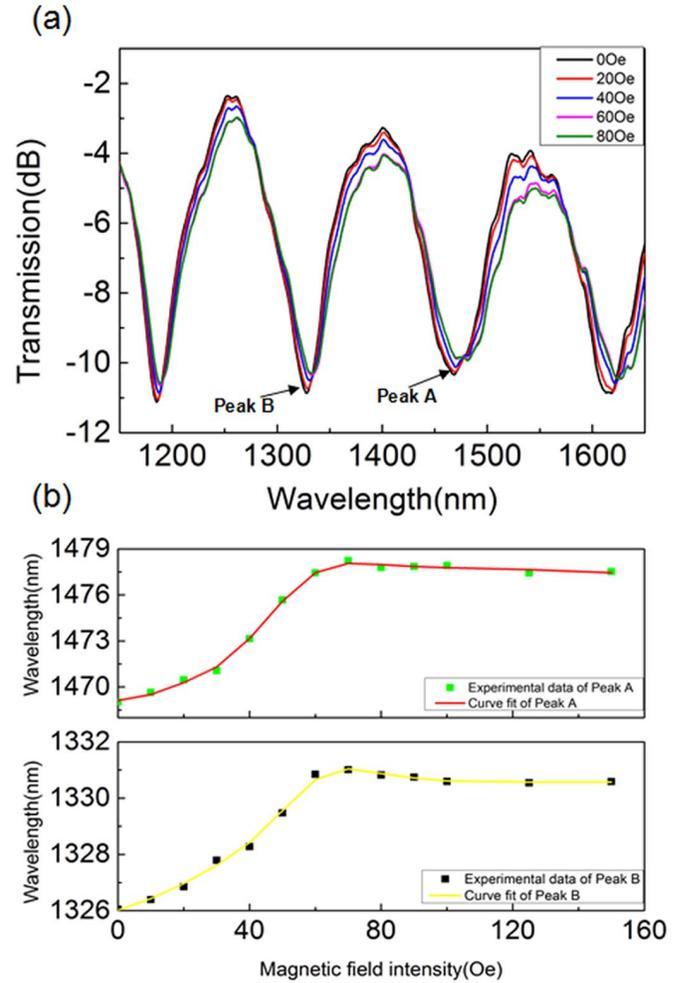
Fig. 2. (a) Transmission spectra of the magnetic fluid-sealed OMT under different magnetic fields intensity. (b) Relationships between magnetic fields intensity and wavelength shift of the resonant peaks.
